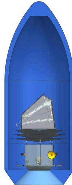
**Figure 4-3.** CDIM fits within EELV dynamic fairings and its bottom V-groove can be reduced in size to fit additional vehicles with minimal impact to instrument thermal performance.
