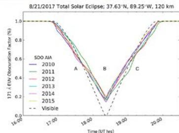
Simulated occultation of the sun at times corresponding to the upcoming 2017 solar eclipse: (A) 17:30 UT, (B) 18:22 UT, and (C) 19:15 UT. Using various years of SDO observations at 171 Å (at 37.63° N, 270.75° E, 125 km), eclipses were simulated. The figure shows the resulting time histories of normalized obscuration factors. Credit: NRL, Huba and Drob 2017
