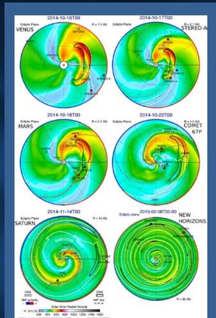
Stills of the solar wind velocity in the ecliptic plane from a CCMC model simulation showing the CME propagation, at the times of the CME's closest approach to Venus, STEREO-A, Mars, comet 67P, Saturn, and New Horizons. The full simulations are available at <http://ccmc.gsfc.nasa.gov>; run numbers Leila\_Mays\_092716\_SH\_1 and Leila\_Mays\_100116\_SH\_1. Credit: Witasse, et. al. (2017).
