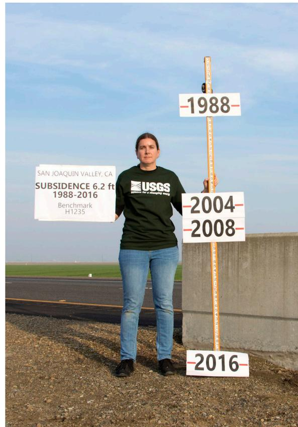
Photograph taken by Justin Brandt, USGS, of the National Geodetic Survey vertical control benchmark H1235 RESET in Merced County, California.
